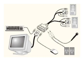
**Step 6** Connect each of the built-in KVM cables to a computer's video and usb ports. You can also connect the cables to the computer's audio and microphone ports.
